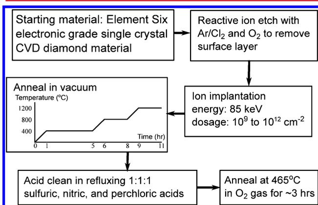
**Figure 1.** Procedure for creating spectrally stable NV centers through ion implantation, annealing, and surface treatment. The Ar/Cl<sub>2</sub> (O<sub>2</sub>) etch was done using an ICP power of 400 W (700 W), a RF power of 250 W (100 W), a DC bias of 423 V (170 V), a chamber pressure of 8 mTorr (10 mTorr), and a gas flow rate of 25/40 sccm (30 sccm). The sample temperature was set to 17 °C.
