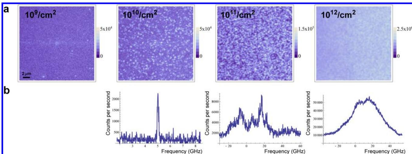
**Figure 2.** (a) Confocal PL images of the implanted layer of NV centers for four different nitrogen ion doses. (b) Corresponding representative PLE spectra for the three highest doses. Each spectrum is the average of  $\sim 10$  PLE scans.
